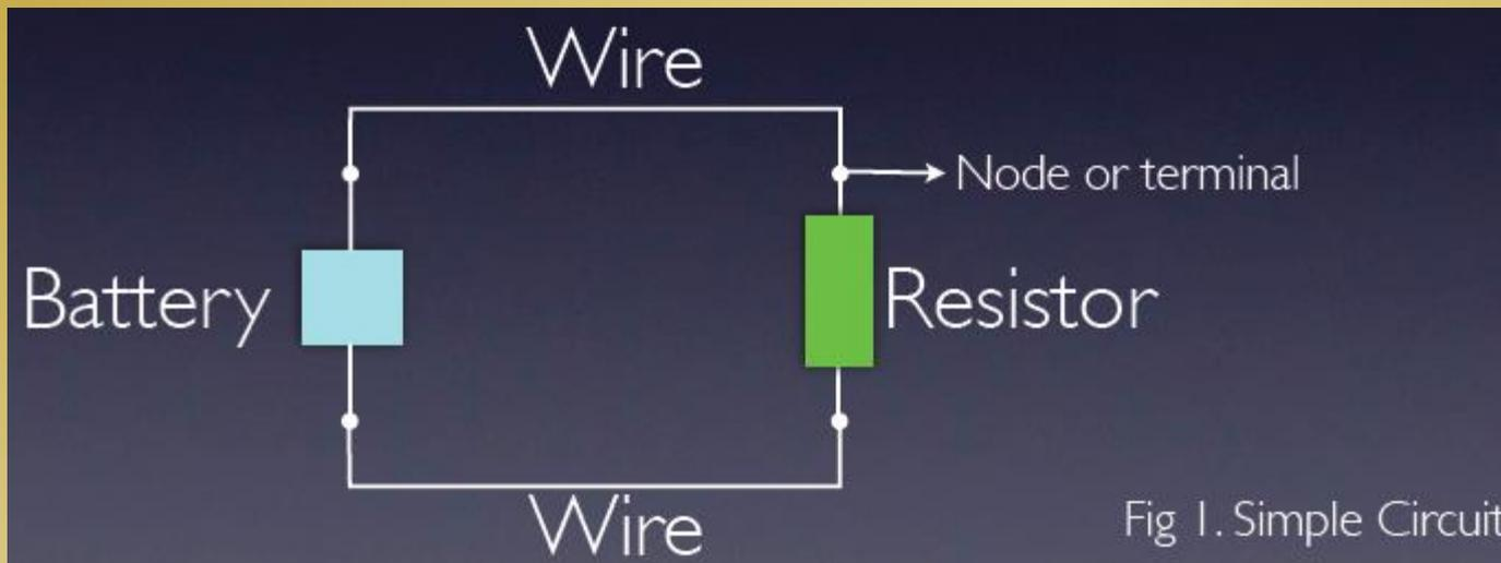
Fig 1. Simple Circuit
