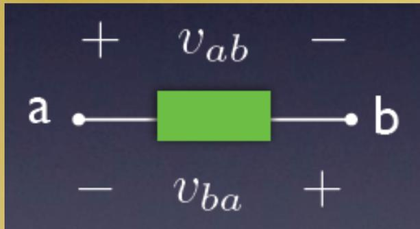
$V_{ab}$  Voltage at terminal a with respect to terminal b
