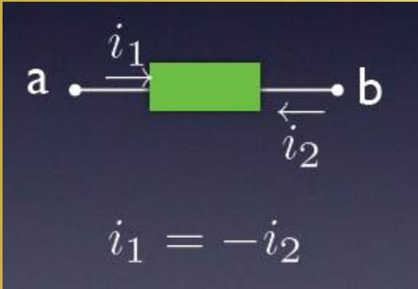
$\vec{i}_1$  → Rate of flow of charge form **node a to node b**
