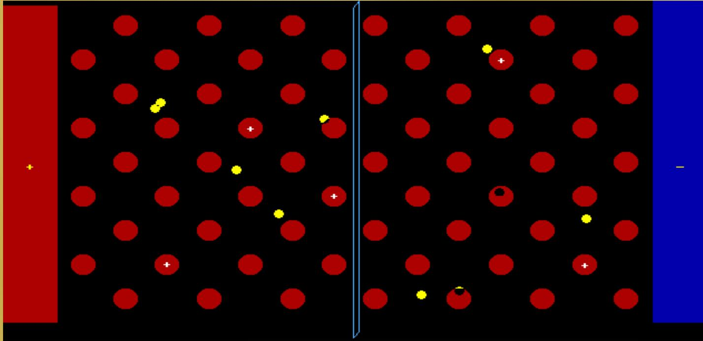
The above animation shows the electrons (yellow) flowing through a conductor. The conventional flow of electrons is from a positive charge towards a negative. This direction of flow was assumed, long before there was any method to check the actual direction the electrons moved in. We now know the electrons do actually flow from the negative to the positive.
